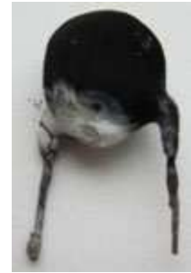
Fig. 6.5.5 MOV Destroyed by Fire
