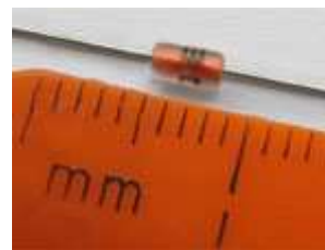
Fig. 6.3.5 DB3 Diac & Circuit Symbol
