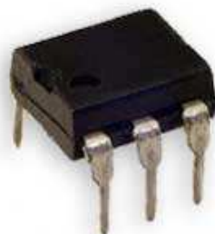
Fig. 6.6.4 Using a MOSFET Relay chip for switching A.C. or D.C.
