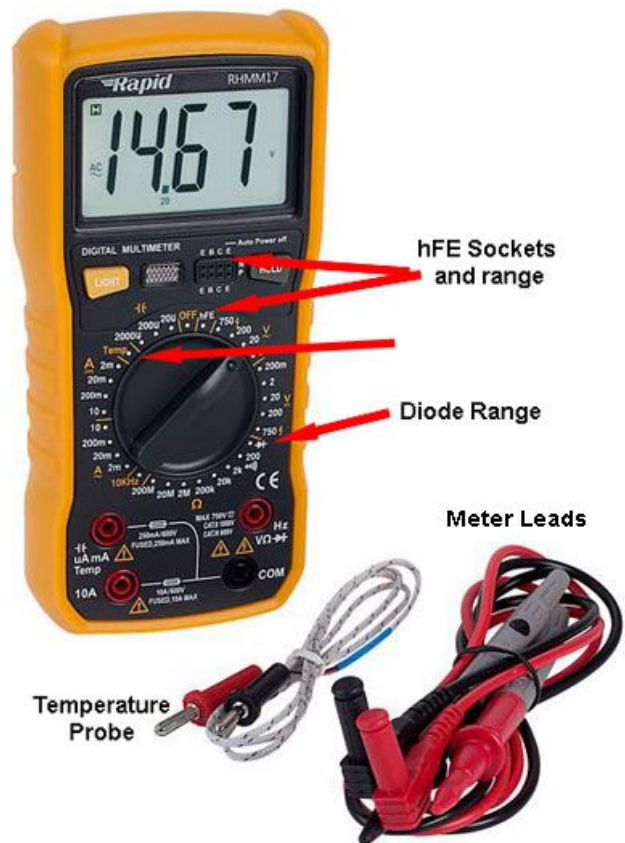
Fig. 7.2.1 Digital Multi-meter with semiconductor testing features.
