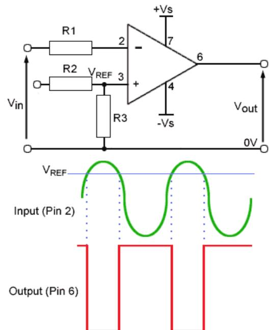
**Fig. 6.6.1 Using an Op Amp as a Comparator**
