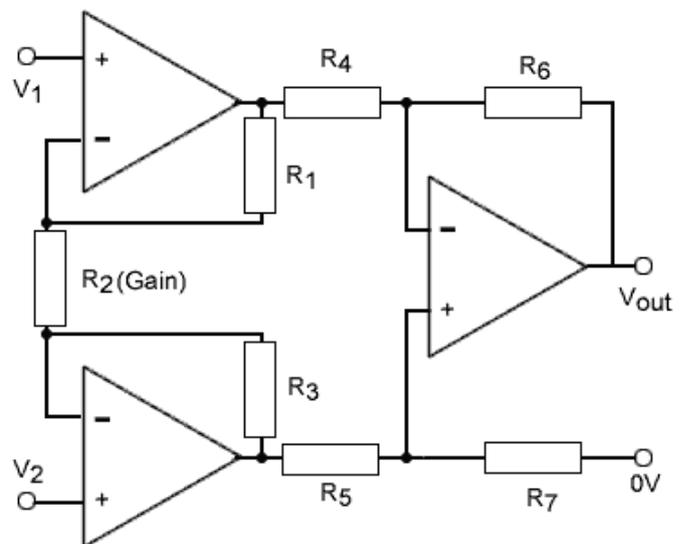
Fig.6.6.3 The Instrumentation Amplifier
